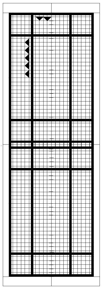
Cut the three sided chips for part of the Diamond border. When making this border, always take the chip next to the centerline first and work out to the end. If you do not do it this way, the diamond pattern will not work.
